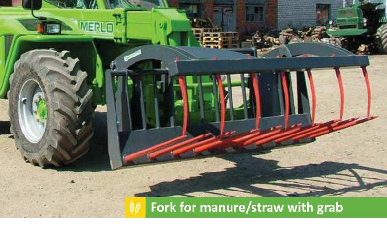
Designed to handle manure with straw content having a maximum density of  $800 \ kg/m^3$
